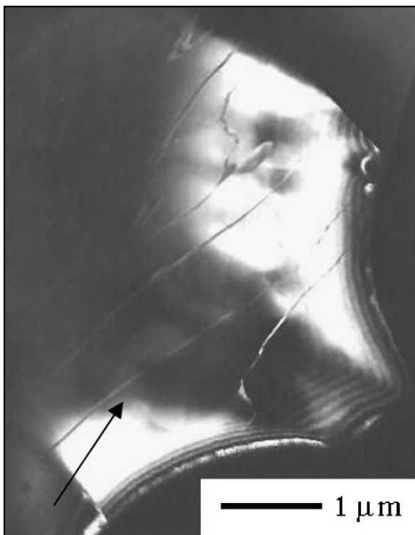
Fig. 5. Dark field (DF) image obtained using a 1/2\{h00\} reflection revealing planar defects with ribbon like morphology (APBs) (arrowed).
